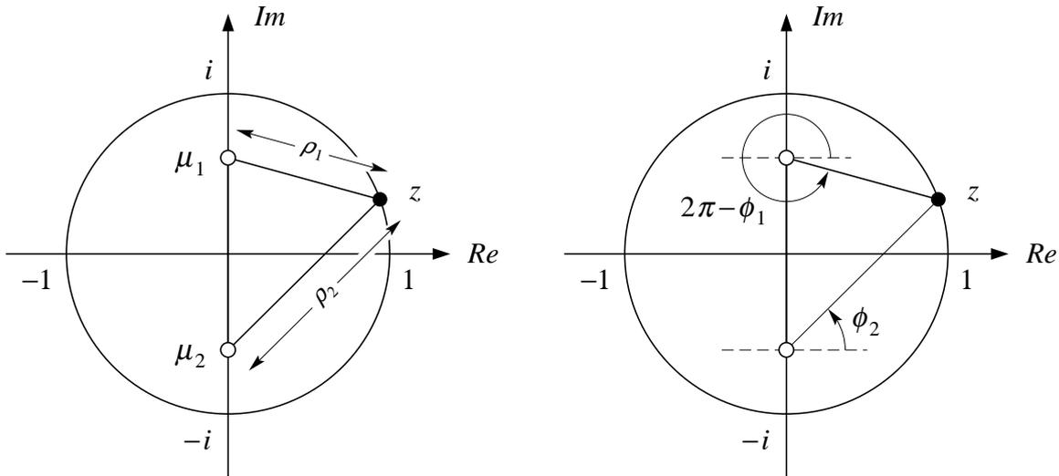
**Figure 7.** The pair of conjugate zeros  $\mu_j, j = 1, 2$  are evaluated at the point  $z = e^{i\omega}$  on the unit circle by finding the moduli  $\rho_j = |z - \mu_j|$  and the arguments  $\phi_j = \text{Arg}(z - \mu_j)$  of the corresponding factors.
